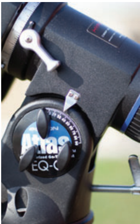
Image 4 –DSP’s Latitude Adjustment Upgrade installs three large thumb bolts that firmly lock a pressure plate at the latitude hub.
